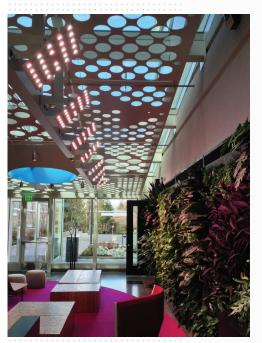
Lighting grow walls can be tricky, says Fong. And this project, which included a massive three-story living wall, posed a particular challenge. Even though a skylight in the space offered some illumination, careful analysis indicated that additional light would be required to keep the plants healthy and thriving. "We knew we'd have to provide a supplemental light source," she says.
